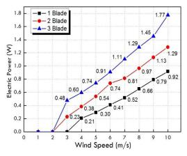
Figure 5:.Output power of wind power generator according to wind speed
