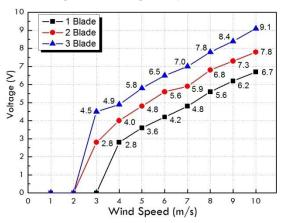
Figure 2: Output voltage of wind power generator according to wind speed
