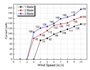
Figure 3: Output current of wind power generator according to wind speed
