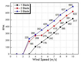
Figure 4: RPM of wind power generator according to wind speed
