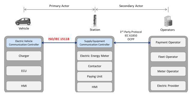
Figure 1: Scope of ISO / IEC 15118 Electric Vehicle Infrastructure Standard
