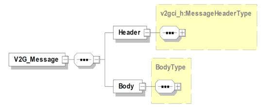
Figure 2: V2G Message scheme of ISO / IEC 15118
