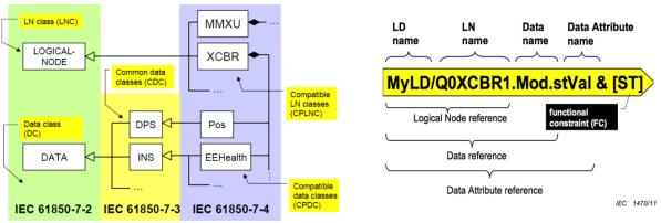
Figure 3: Data stack and Data representation method of IEC 61850
