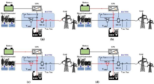
Figure 3:. Proposed Uninterruptible hybrid CTTS System Operating Modes
