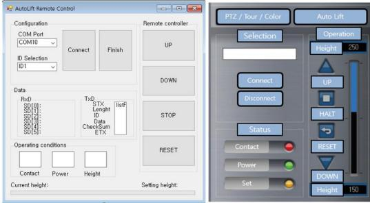
Figure 4: ALS control program a) Independent type b) NVR-integrated type
