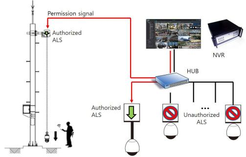
Figure 3:.ALS and CCTV cameras controlled by NVR
