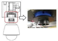
Figure 5:.Lower socket detached inside the ALS
