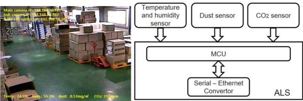
Figure 6:.Display of data from sensors on screens and sensor hardware composition using ALS
