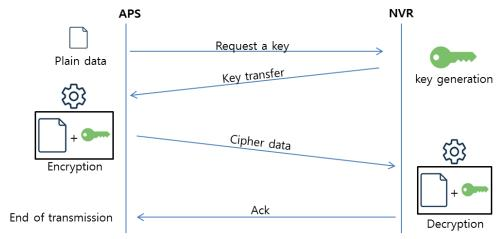
Figure 7:. Communication procedure between ALS and NVR using encrypted key
