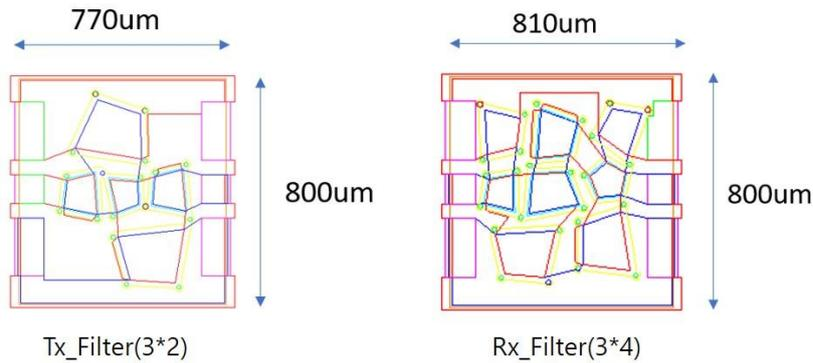
Figure 8: Design for Tx, Rx Filters
