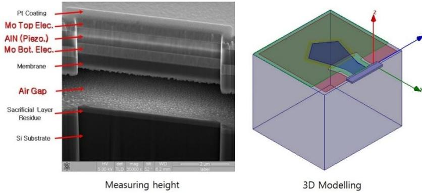
Figure 1.: 3D Modelling and SEM image of fabricated FBAR
