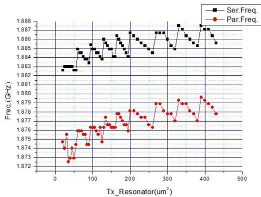
Figure 3.: Frequency deviation by resonator size
