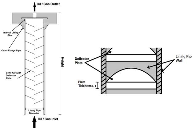
Fig. 1: Nomenclature of a stand pipe and deflector plate
