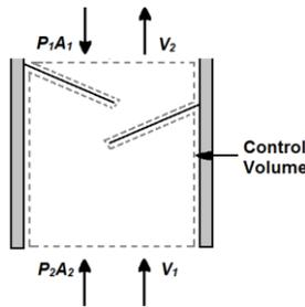
Fig. 3: Pressure drop across the stand pipe
