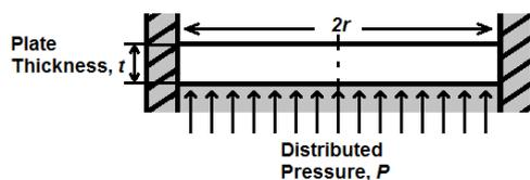
Fig. 4: Circular plate stress and deformation parameters
