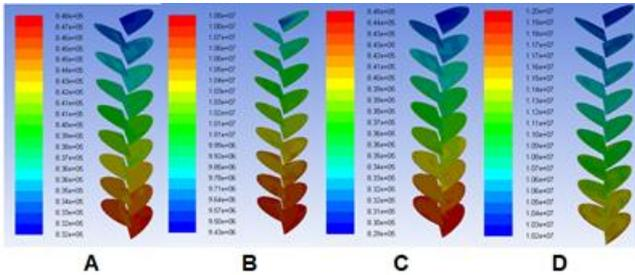
Fig. 5: Absolute pressure contour on deflector plate
