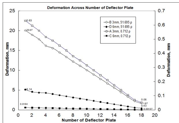
Fig. 9: Deformation across Number of Plate
