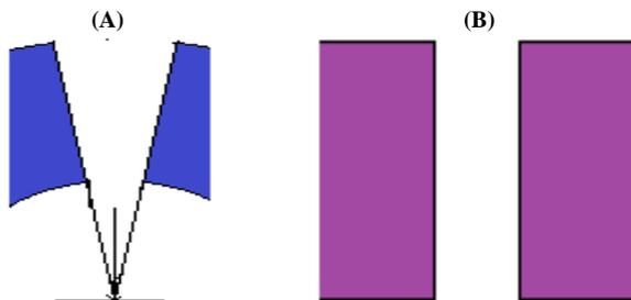
Fig. 4: Unskewed Rotor Poles (A) Axial Poles (B) Radial Poles
