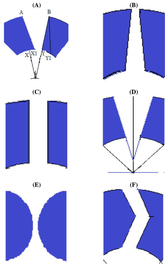
**Fig. 6:** Axial Rotor Magnet Skewing (A) Conventional Skewing (B) Triangle Shape Skewing (C) Parallel Skewing (D) Trapezoid Type Skewing (E) Round Shape Skewing (F) Dual Skewing.
