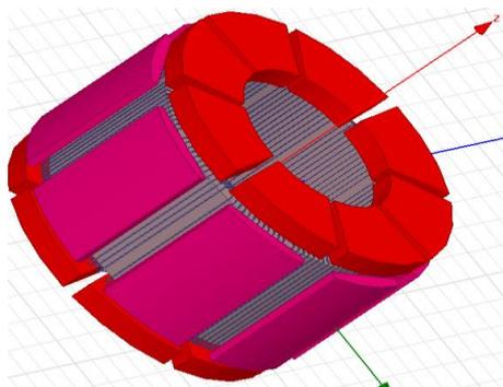
Fig. 2: 3D Radial and Axial Rotor and Inner TS Stator.
