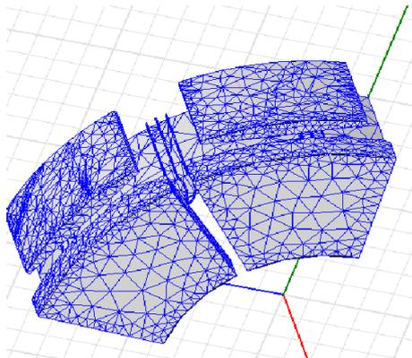
Fig. 3: 3D Section of Both Radial and Axial Rotor and Stator Meshed in FEM.
