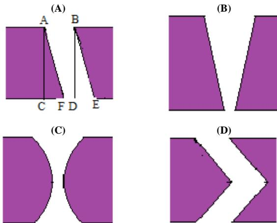
Fig. 7: Radial Rotor Magnet Skewing. A) Parallel Skewing B) Triangular Skewing C) Round Skewing and D) Dual Skewing.
