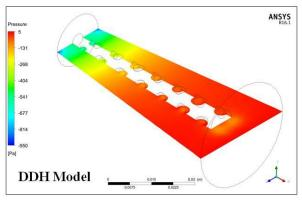
Fig. 10: Static pressure contour for the divergent dimple hub (DDH)
