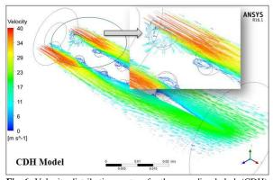
Fig. 6: Velocity distribution vectors for the cone dimple hub (CDH)
