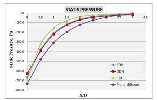
Fig. 12: Comparison of the static pressure profile for annular diffuser fitted with SDH, DDH, CDH and Plane diffuser
