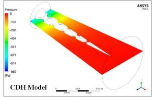
Fig. 11: Static pressure contour for the cone dimple hub (CDH)
