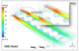
Fig. 4: Velocity distribution vectors for the straight dimple hub (SDH)
