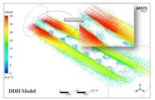
Fig. 5: Velocity distribution vectors for the divergent dimple hub (DDH)
