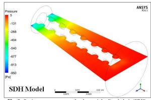
Fig. 9: Static pressure contour for the straight dimple hub (SDH)
