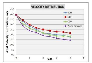
**Fig. 8:** Comparison of the axial velocity profile for annular diffuser fitted with SDH, DDH, CDH and Plane diffuser
