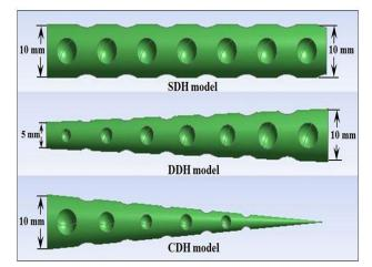
Fig.2: Different dimpled hub models
