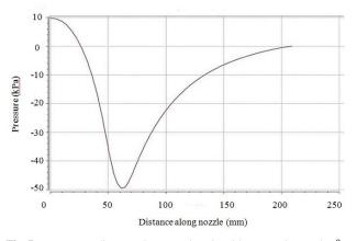
**Fig. 7:** Pressure vs distance along nozzle axix with converging angle,  $\theta_1 = 18^\circ$  and inlet hole position, X = 59.5 mm
