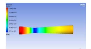
Fig. 6: Pressure contour for nozzle with converging angle,  $\theta_1 = 18^\circ$  and inlet hole position, X = 59.5 mm
