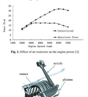
Fig. 2: Example of Formula SAE car engine restrictor system [3]
