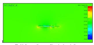
Fig 14: Pressure Contour at 7° angle of attack, Case
