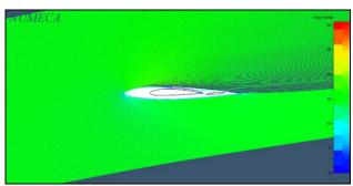
Fig 17: Velocity profile at  $11^{\circ}$  angle of attack, Case II
