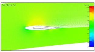
Fig 12: Velocity profile at 7° angle of attack, Case
