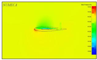
Fig 19: Pressure Contour at 11° angle of attack, Case II
