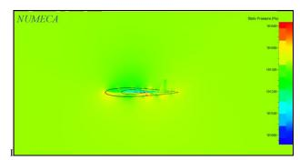
Fig 15: Pressure Contour at 9° angle of attack, Case
