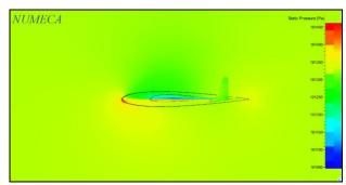
Fig 18: Pressure Contour at 9° angle of attack, Case II
