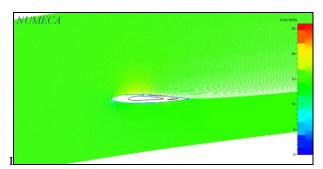
Fig 13: Velocity profile at 9° angle of attack, Case
