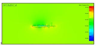
Fig 14: Pressure Contour at 7° angle of attack, Case
