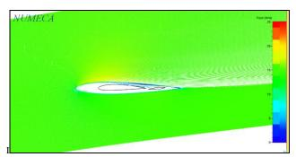
Fig 16: Velocity profile at 9° angle of attack, Case II
