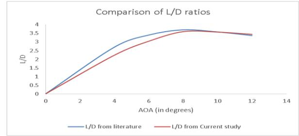
Fig. 5: Comparison of L/D ratio with literature [4]
