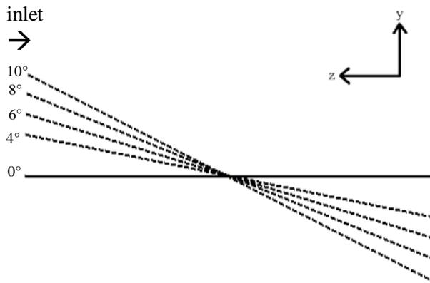
Fig. 4: Left side view of wing oriented at different AoA; solid line represents wing at  $0^\circ$ , dotted lines represent the wing at  $4^\circ$ ,  $6^\circ$ ,  $8^\circ$  &  $10^\circ$  respectively
