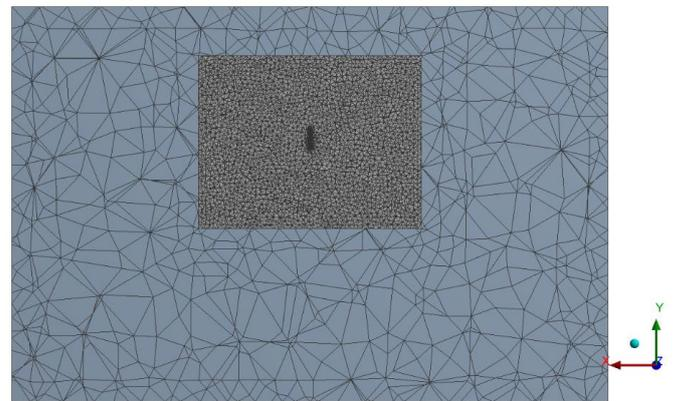
Fig. 3: Meshing of the cuboidal domains; the inner domain has finer meshing than the outer one. Close to the wing the mesh is highly detailed.
