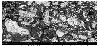
(a) particles size of 125-177  $\mu$ m (b) particles size less than 74  $\mu$ m **Fig. 7:** SEM images of Sokka-clay/Phenolic Composite varied in particle size
