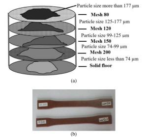
Fig. 1: (a) Scheme of sieving process and (b) tensile test sample
