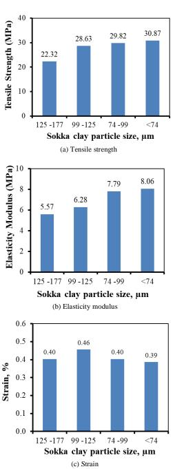
Fig. 5: Tensile properties of Sokka-clay/phenolic composite varied in particles size
