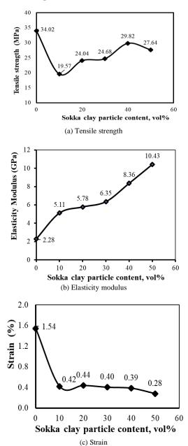
Fig. 4: Tensile properties of Sokka-clay/phenolic composite varied in particle content
