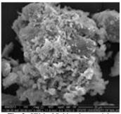
Fig. 2: SEM of Sokka clay particle
