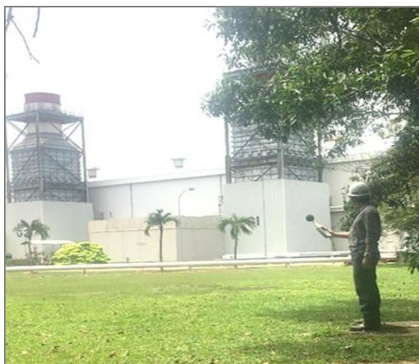
Fig 3: In-situ Noise Measurement Setup
