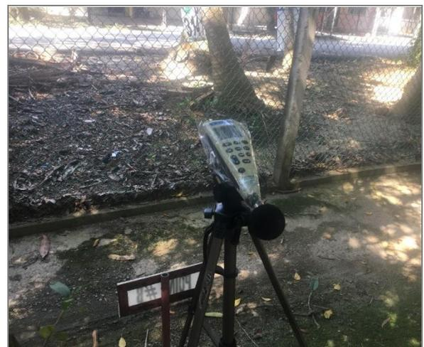
Fig2: Continuous Noise Monitoring Set up
