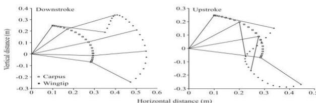
Fig. 2: Folding in and out motion of a bat wing during flight [5].
