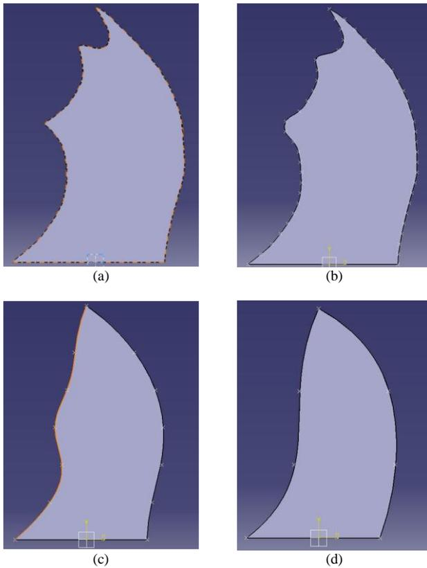
**Fig. 4:** Generated wing geometry where; (a) is the 99 vertices wing, (b) is the 49 vertices wing, (c) is the 13 vertices wing, and (d) is the 7 vertices wing
