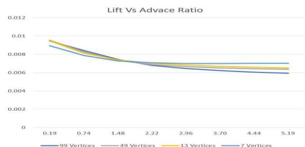
**Fig. 6:** Advance ratio Versus Averaged lift generated
