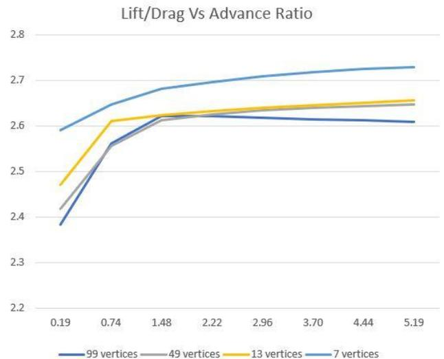
Fig. 8: Aerodynamic Efficiency, Lift/Drag Versus Advance Ratio
