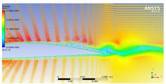
Fig. 10: Velocity vector for NACA 4415
