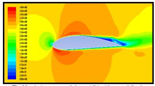
Fig. 14: velocity contour at 0 degree AOA with outward dimple
