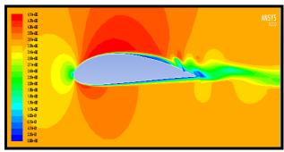
Fig. 13: velocity contour at 0 degree AOA with inward dimple
