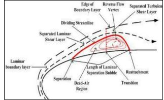
Fig. 1: Laminar Separation Bubble [1]
