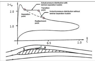
Fig. 2: Pressure distribution over airfoil with LSB [2]
