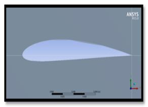
Fig. 6: Geometry of NACA 4415 aerofoil created in ANSYS
