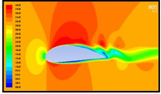
Fig. 12: velocity contour at 0 degree AOA without dimple
