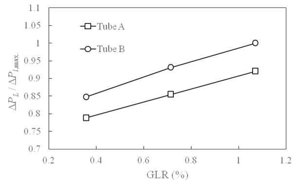
**Fig. 8:** Normalized liquid pressure drop plotted against GLR for aeration tubes as indicated.
