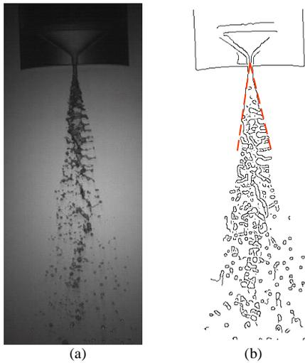
**Fig. 3:** Typical swirl spray for measurement of spray angle. (a) original image and (b) spray edges using Canny Edge Detection algorithm.
