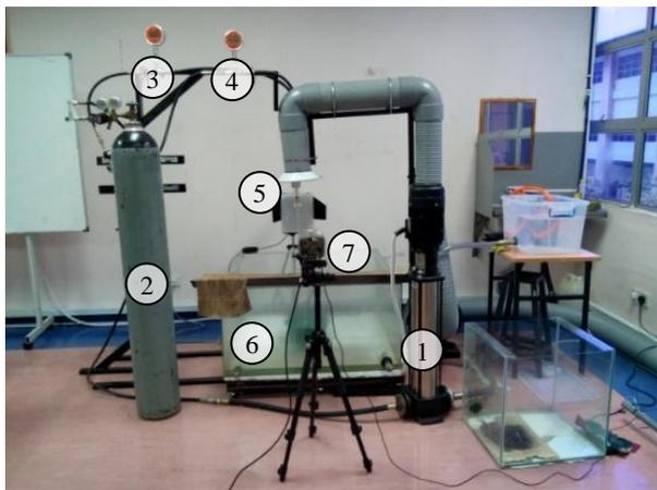
Fig. 1: Experiment test rig for atomizer cold flow test
