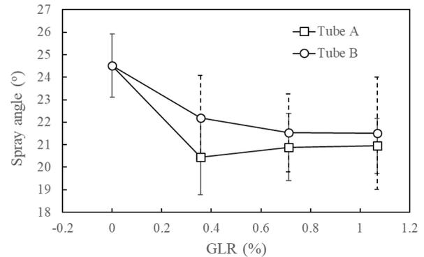
**Fig. 4:** Average spray angle plotted against GLR for aeration tubes as indicated. Error bars represent standard deviations of the mean spray angle.
