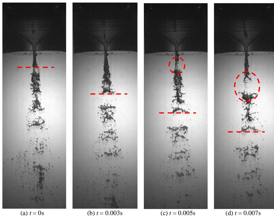
**Fig. 5:** Development of typical swirl effervescent atomization. Photos were taken for atomizer I at  $\text{GLR} = 0.36\%$ . Dashed lines represent the front-end of the liquid sheet, indicating progression of flow with time.
