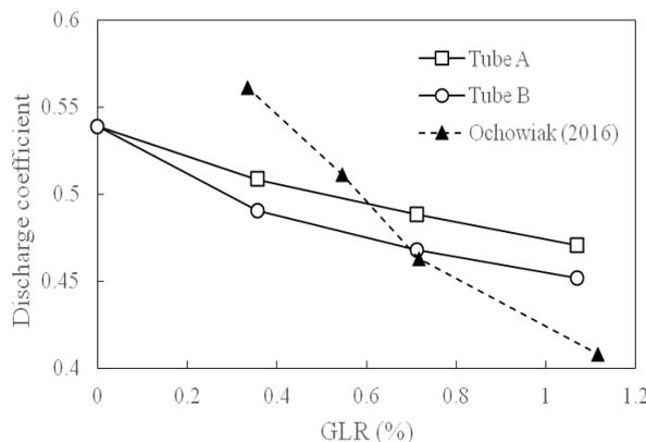
**Fig. 7:** Discharge coefficient plotted against GLR for aeration tubes as indicated.
