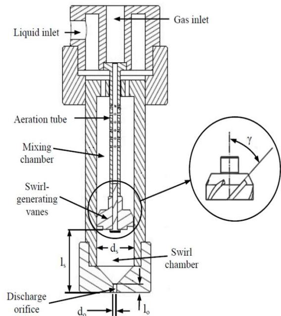
Fig. 2: Schematic of swirl effervescent atomizer
