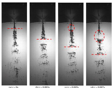
Fig. 5: Development of typical swirl effervescent atomization. Photos were taken for atomizer I at GLR = 0.36%. Dashed lines represent the front-end of the liquid sheet, indicating progression of flow with time.
