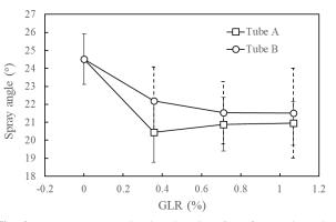
Fig. 4: Average spray angle plotted against GLR for aeration tubes as indicated. Error bars represent standard deviations of the mean spray angle.
