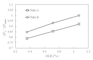
Fig. 8: Normalized liquid pressure drop plotted against GLR for aeration tubes as indicated.
