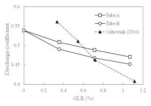
Fig. 7: Discharge coefficient plotted against GLR for aeration tubes as indicated.
