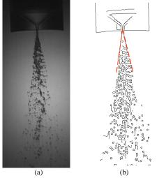
Fig. 3: Typical swirl spray for measurement of spray angle. (a) original image and (b) spray edges using Canny Edge Detection algorithm.
