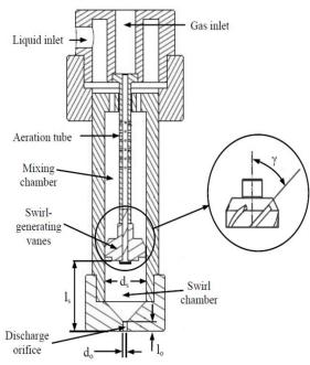
Fig. 2: Schematic of swirl effervescent atomizer
