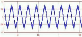
Fig.10: Current output of inverter after current controller implementation
