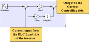
Fig.5: PI Controller block in MATLAB-Simulink
