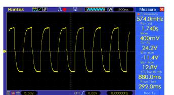
Fig 12: Output of the inverter with current control with filter
