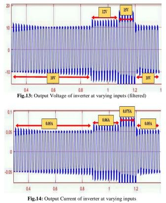
Figs. 13 and 14 show the results which have been displayed in GUI during RCP process as example for the voltage output of the inverter whenever the input voltage is changed. The changed are immediate and followed the PI control response and it has very minor down-time which is approximately of 20ms. At the mean-time, the current waveform output follows the voltage changes in instant mode which enables the PWM to generate smoothly with current close-loop system in real time mode
