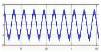
Fig.9: Voltage output of inverter after current controller implementation
