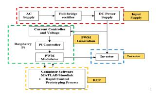
**Fig.1:** Block diagram for Rapid Control Prototyping of a single-phase back to back converter for a single phase network
