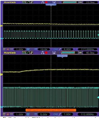
Fig.11: Output of the PWM signals to the inverter with current control
