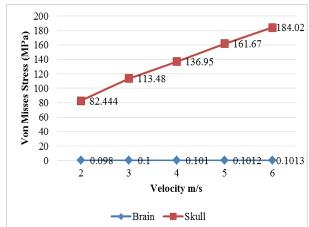
Figure 3: Stress distribution (von misses) in skull and brain at different velocity.
