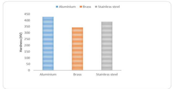
Fig. 8: Microhardness of CoNiFe coated on aluminium, brass and stainless steel
