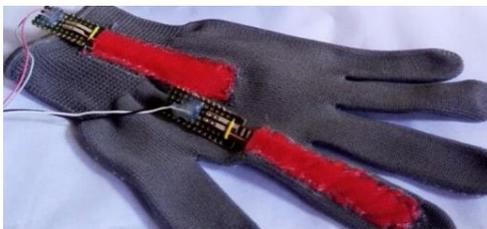
Figure 3: Resistive flex sensor mounted on the glove
