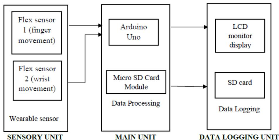
Figure 1: Block diagram of post stroke rehabilitation system
