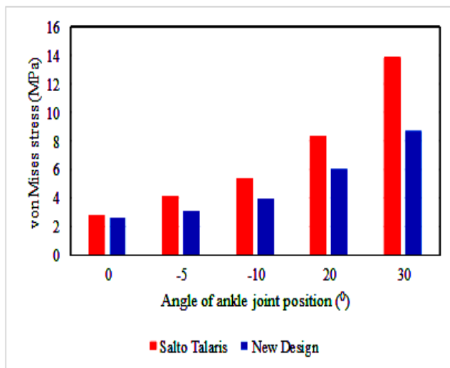
Fig. 4: The von Mises stress at PE insert versus ankle joint flexion angle.
