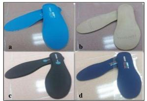
**Fig.3:** Four different insole material used in the study; (a) EVA insole, (b) PU insole, (c) Polyester insole and (d) PU Gel insole
