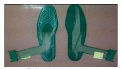
Fig.2: The FScan sensor
