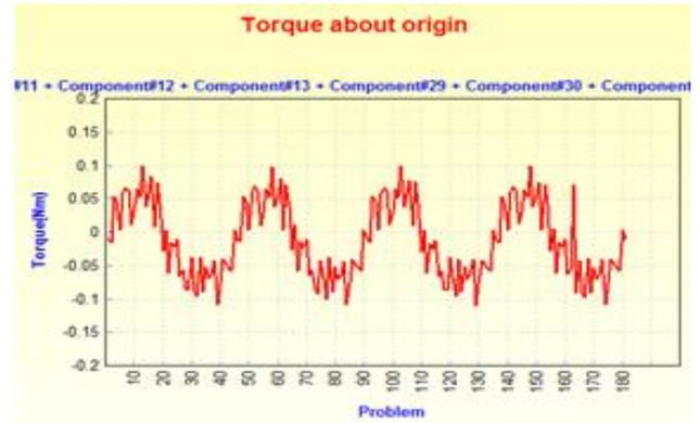
Fig. 5: Cogging Torque
