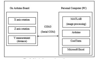
Fig. 2: Block diagram of overall system.
