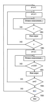
Fig. 6: Control algorithm flow in the Arduino hardware platform.
