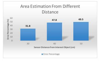
Fig. 9: Error percentage obtained from different distances between sensor and object of interest.
