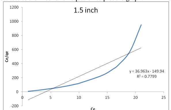
Fig. 1: Langmuir Isotherm Model for 1.5 inch of EFB-HBC
