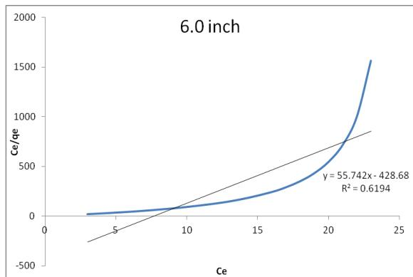
Fig. 3: Langmuir Isotherm Model for 6.0 inch of EFB-HBC
