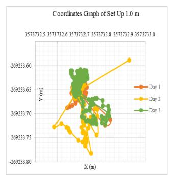
Changing the antenna height will change the point of antenna phase centre thus causing a slight different in coordinates obtained.
