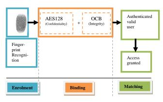
Fig. 5: Conceptual Model of Biometric Fingerprint Template Protection
