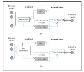
**Fig. 4:** The Basic Concept of Biometric Encryption (a) Key Binding and (b) Key Generation [11]
