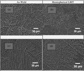
**Fig. 3:** Microstructure changes of (a) HAZ as-welded, (b) HAZ 20 Joule LBIT (c) fusion zone as-welded and (d) fusion zone 20 Joule LBIT
