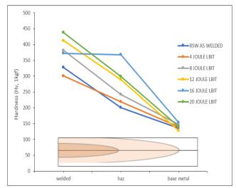
Fig. 6: Hardness profile of the samples.
