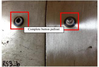
Fig. 4: Failure mode of 20 Joule LBIT samples.
