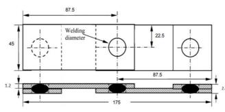
Fig. 1: Spot welding sample dimension
