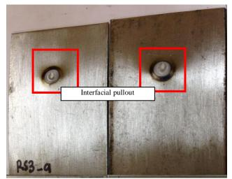
Fig. 5: Failure mode of 4 Joule LBIT samples
