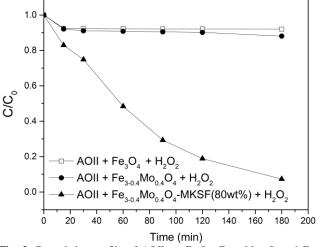
Fig. 3: Degradation profile of AOII on  $Fe_3O_4$ ,  $Fe_{3^-0.4}Mo_{0.4}O_4$  and  $Fe_{3^-0.4}Mo_{0.4}O_4$ -MKSF(80wt%) in catalytic test. Experimental conditions: AO7 35 mg/L,  $H_2O_2$  20mM, catalyst 0.1g/L and pH 3.
