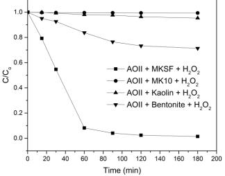
Fig. 1: Degradation profile of AOII on MKSF, MK10, Kaolin and Bentonite in catalytic test
