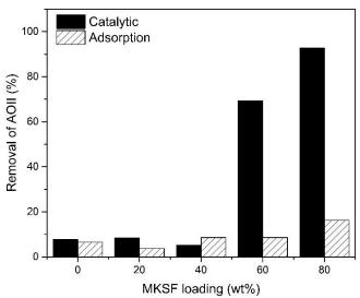
Fig. 2: AOII removal by adsorption catalytic Fenton-like reaction using  $Fe_{3^{-}0.4}Mo_{0.4}O_4$  catalyst at varies MKSF loading (wt%)
