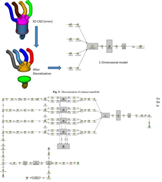
Fig. 4: Complete 1-D model of the engine
