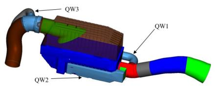
Fig. 6: Air intake module of a baseline 1600cc engine
