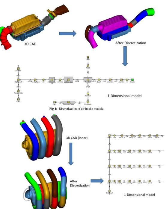
Fig 2: Discretization of intake manifold
