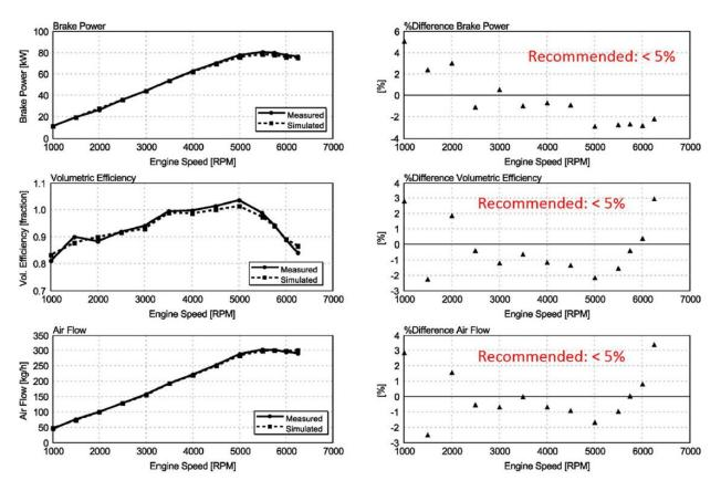
Fig. 5 Engine Performance Model Correlation
