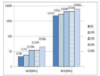
Fig. 1: Effect of strands ratio on the MOR and MOE of rice husk particleboard  $% \mathcal{A} = \mathcal{A}$
