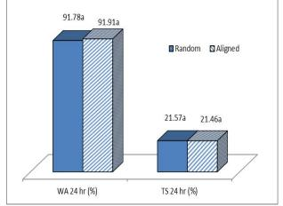
Fig. 4: Dimensional stability properties of rice husk particleboard for *A*. *excelsa* strands arrangement
