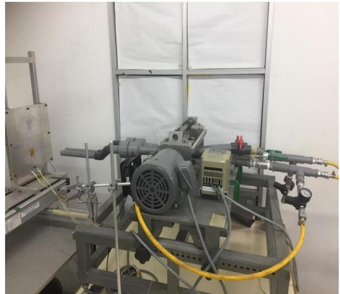
Fig. 4: Twin Impingement jets Mechanism and heat flux microsensors on the Aluminium impingement surface.
