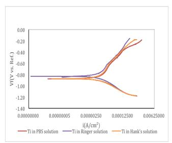
Fig. 1: Polarization curves for Ti-6Al-4V in SBF
