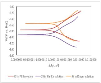
Fig. 2: Polarization curves for 316L SS in SBF
