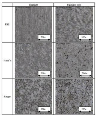
Fig. 5: Microstructure of Ti-6Al-4V and 316 SS in SBF
