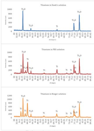
Fig. 3: XRD for Ti-6Al-4V in SBF
