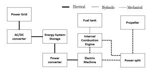
Fig. 3: Block diagram of the proposed PHERB powertrain
