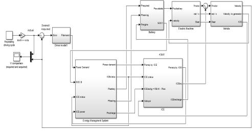
Fig. 4: Overall structure of the PHERB model in MATLAB/SIMULINK
