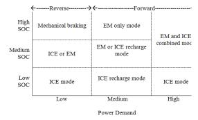
Fig 5: PHERB EMS modes of operation.
