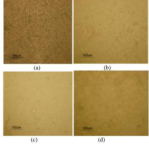
Fig 1: Optical microscopy for Ti-6Al-4Vally (a) uncoated & (b, c, and d) coated with  $\text{TiO}_2$  for different thicknesses.
