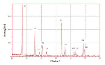
Fig 3: X-ray diffraction for titania  $TiO_2$  (thickness 58  $\mu$ m) coated Ti-6Al-4V allov.
