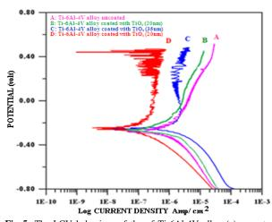
Fig 5: The LCV behaviour of the of Ti-6Al-4V alloy (a) uncoated, (b) coated with  $TiO_2$  (thickness 20  $\mu$ m), (c) coated with  $TiO_2$  (thickness 35  $\mu$ m), (d) coated with  $TiO_2$  (thickness 58  $\mu$ m).
