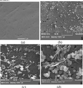
**Fig 4:** Top view of the SEM of Ti-6Al-4V alloy (a) uncoated, (b) coated with  $TiO_2$  (thickness 20  $\mu$ m), (c) coated with  $TiO_2$  (thickness 35  $\mu$ m), (d) coated with  $TiO_2$  (thickness 58  $\mu$ m).
