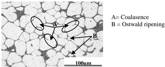
**Fig 8:** Close-up microstructure of Al-5.7Si-2Cu-0.3Mg alloys after reheating trial at 600 °C.
