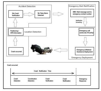
Fig 3: The Proposed Framework Interacting Component
