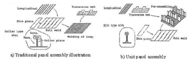
Figure 3: Comparison between modular Construction and conventional Shipbuilding [5] [9].
