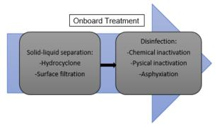
Fig. 1: Ballast Water Treatment Onboard Ship
