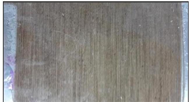
**Fig. 2 :** Cured Kenaf Composite plate
