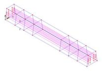
Fig. 4: Line model of monoblock prestressed concrete sleeper and prestressing tendon
