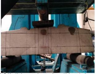
Fig. 7: Monoblock prestressed concrete sleeper with the reaction frame (Positive Moment Test)
