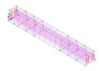
Fig. 5: The meshed volume of monoblock prestressed concrete sleeper and meshed line of prestressing tendon
