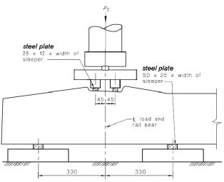
**Fig. 6:** Rail seat – Positive Moment Test, Repeated Load Test, Bond Development and Ultimate Load Test (AS 1085.14 – 2012)
