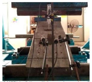
Fig. 8: LVDT is installed in monoblock prestressed concrete sleeper (Positive Moment Test)
