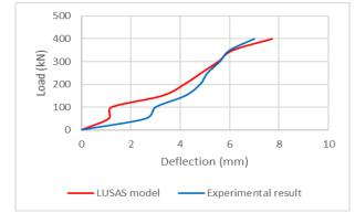
Fig. 13: Comparison of load-deflection between LUSAS Finite Element Model and Experimental Result
