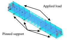
Fig. 10: The assigned attributes on the model of monoblock prestressed concrete sleeper
