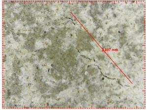
Fig. 9: First crack appeared on the surface of the sleeper
