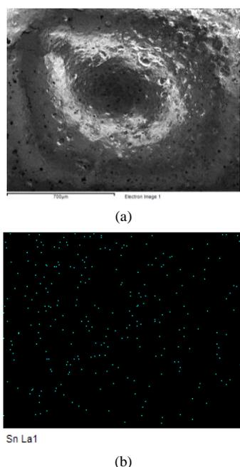
**Fig. 3:** (a) SEM image for coating of ceramic surface using PVA (b) Composition of tin by mapping technique using EDX
