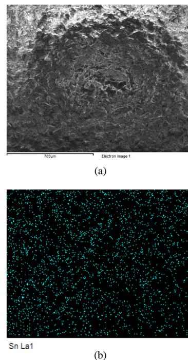
**Fig. 4:** (a) SEM image for coating of ceramic surface using PEG (b) Composition of tin by mapping technique using EDX
