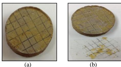
**Fig. 5:** Surface area for PVA (a) before adhesion test and (b) after adhesion test
