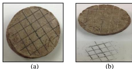
**Fig. 6:** Surface area for PEG (a) before adhesion test and (b) after adhesion test
