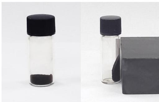
Fig. 7: Magnetic behavior of iron oxide nanoparticles
