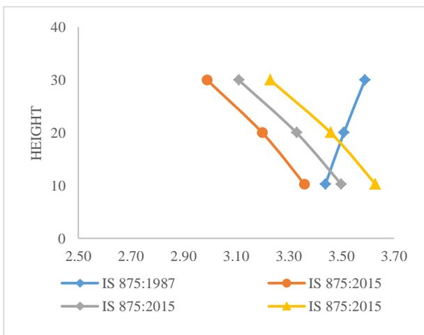
Fig. 8: Variation of gust for 30 m tube monopole tower
