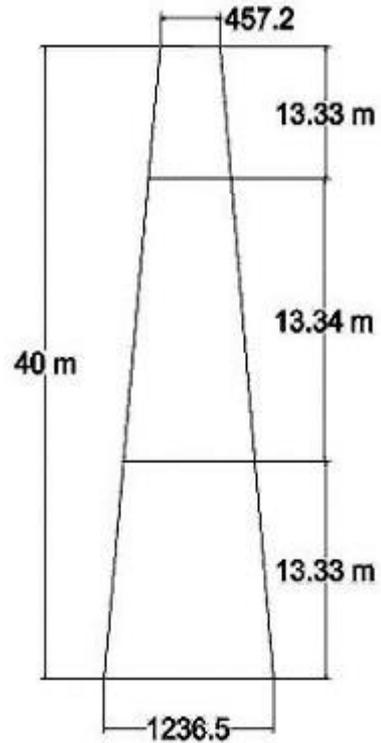
Fig. 3: 40m tube monopole with basic wind speed = 50m/sec.
