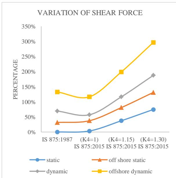
Fig. 20: Shear force variation for 30m tube monopole
