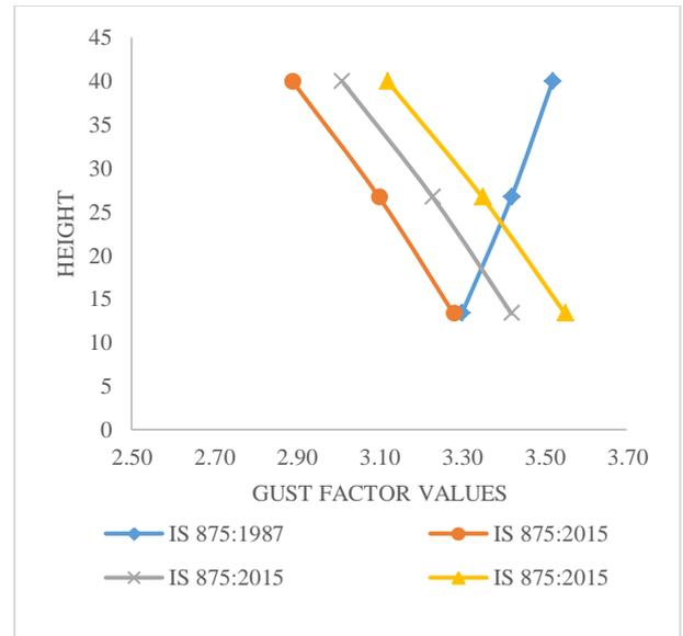
Fig. 10: Variation of gust for 40 m tube monopole tower
