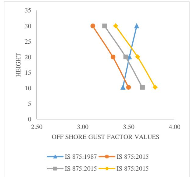
Fig. 9: Variation of gust with offshore for 30 m tube monopole tower
