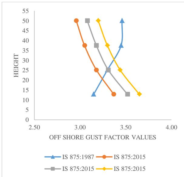
Fig. 13: Variation of gust with offshore for 50 m tube monopole
