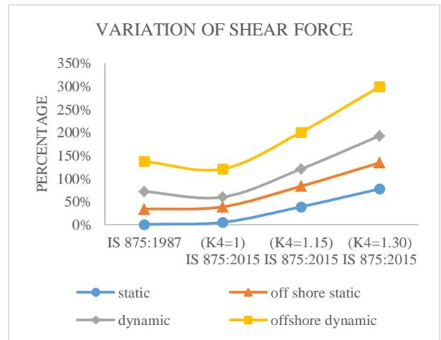
Fig. 28: Shear force variation for 50m tube monopole
