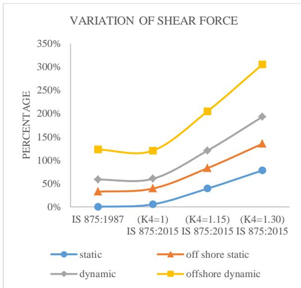
Fig. 24: Shear force variation for 40m tube monopole
