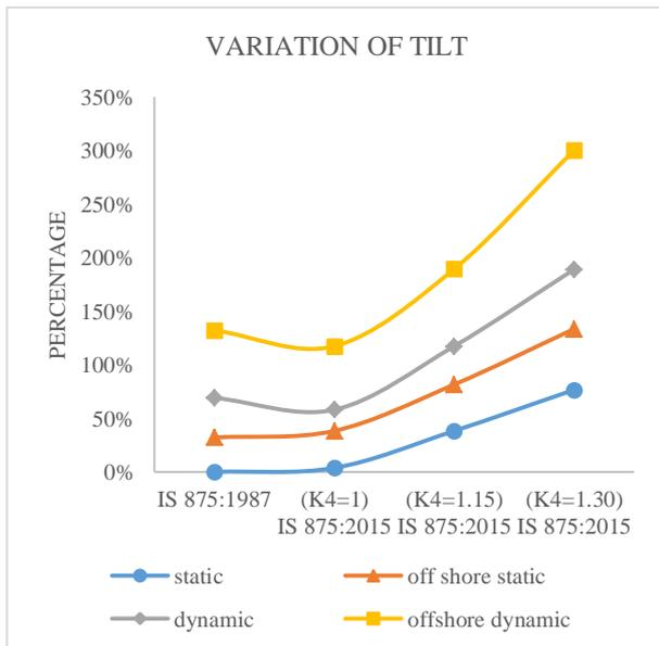
Fig. 25: Tilt variation for 40m tube monopole tower
