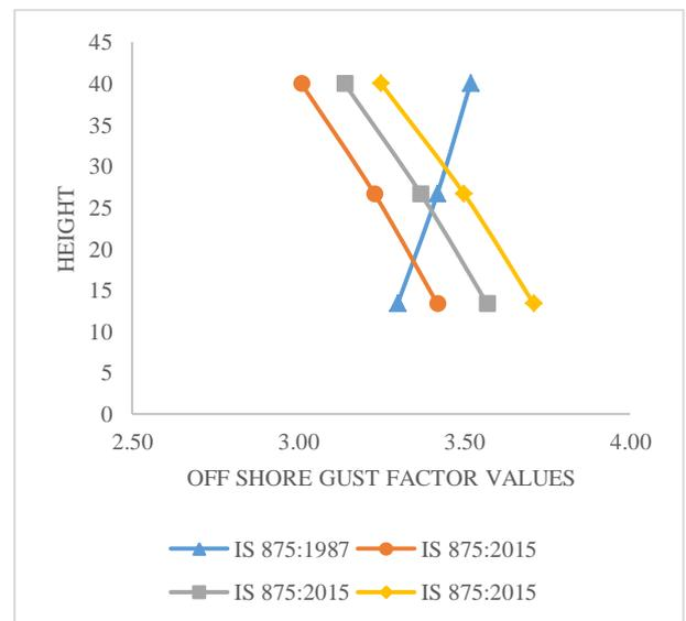
Fig. 11: Variation of gust with offshore for 40 m tube monopole
