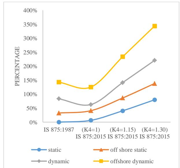
Fig. 16: Shear force variation for 30m pipe monopole
