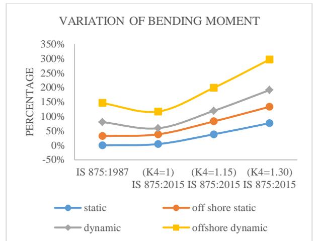
Fig. 27: Bending moment variation for 50m tube monopole
