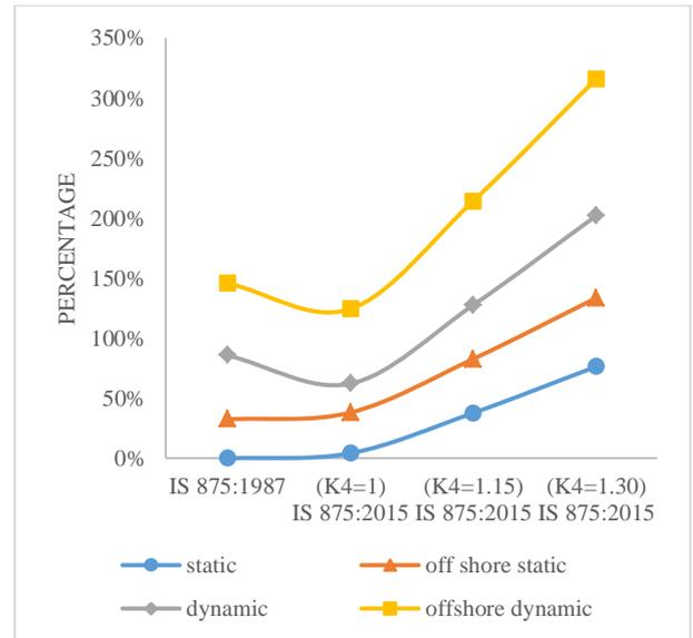
Fig. 15 Bending moment variation for 30m monopole
