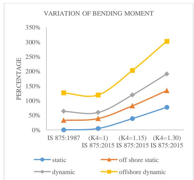
Fig. 33: Bending moment variation for 40m tube monopole
