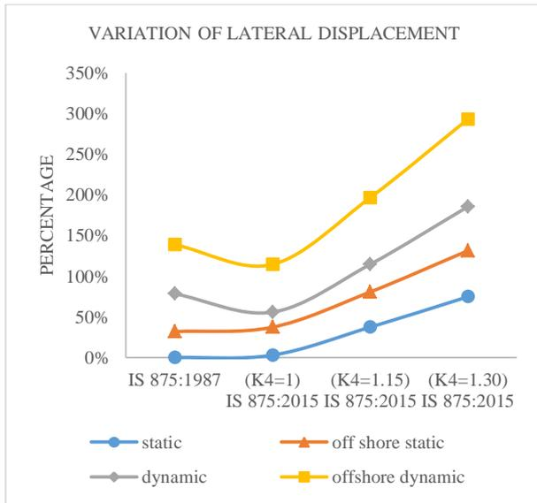
Fig. 18: Lateral displacement variation for 30m tube monopole
