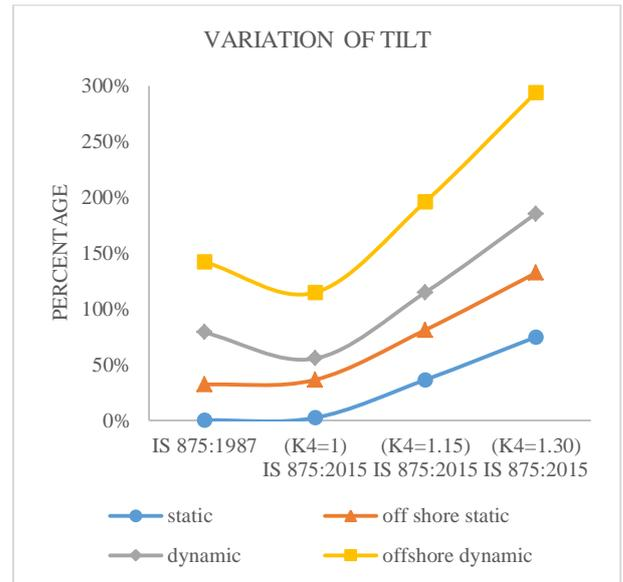
Fig. 21: Tilt variation for 30m tube monopole
