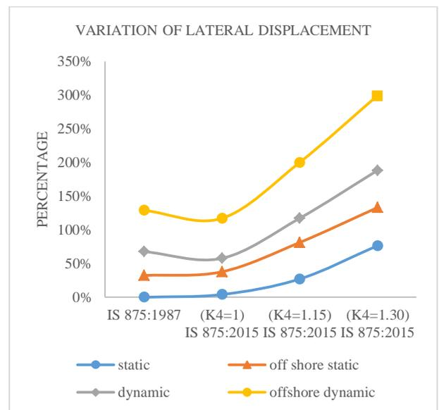
Fig. 22: Lateral displacement variation for 40m tube monopole
