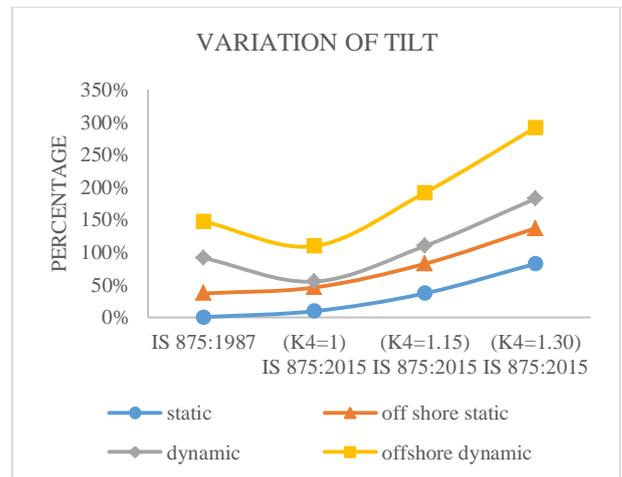
Fig. 29: Tilt variation for 50m tube monopole
