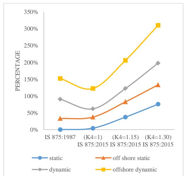
Fig. 17: Tilt variation for 30m pipe monopole
