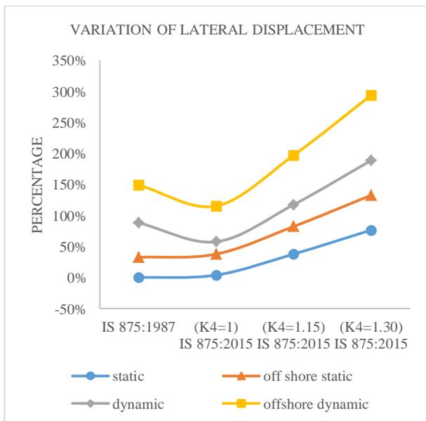
Fig. 26: Lateral displacement variation for 50m tube monopole
