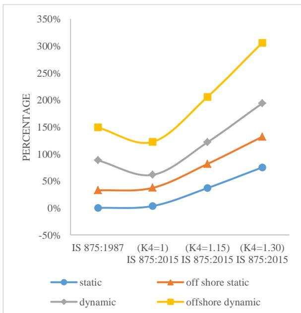
Fig. 14: Lateral displacement variation for 30m pipe monopole
