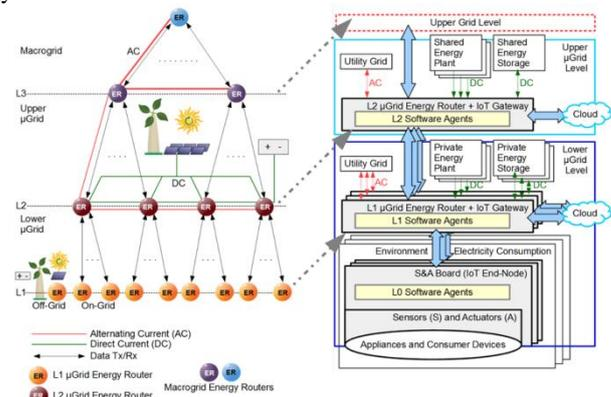
Fig. 1: Simplified architecture of the proposed IoTaaS Energy Management.
