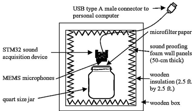
Fig. 2: Audio acquisition setup
