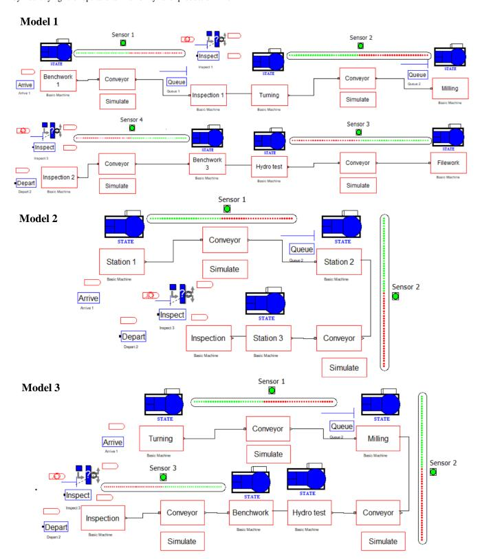
Fig. 2. Configuration layout - Production Simulation Models
