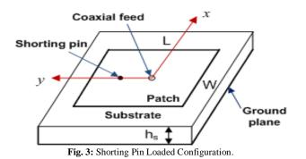
Here by introducing a shorting pin in the patch, the physical size reduction of the MPA has been achieved. A good impedance matching for the dual band frequencies are also achievable. The overall physical size, 63.4 x 60.5 mm2 of the MPA meets the requirement of the RF energy harvester system. The proposed MPA with a single shorting pin is as shown in Fig. 3. The configuration consists of a radiator patch, a shorting pin and a coaxial feed connector that analyzed by transmission line model [15].
