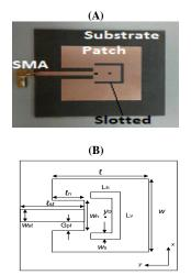
Fig. 2: The A) Fabricated and B) Geometry Layout of the Proposed Design.
