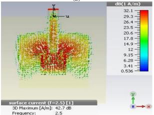
Fig. 7: Simulated Current Distribution at A) 1.8 GHz and B) 2.5 GHZ.
