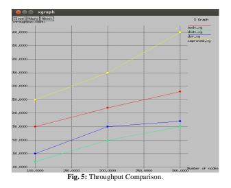
As shown in figure 5, the throughput of the AODV, DSR, DSDV and improved protocol is compared correspond to number of nodes. The throughput increased at steady rate due to generation of efficient path from source to destination. It is analyzed that improved protocol has maximum performance as compared to other protocols.
